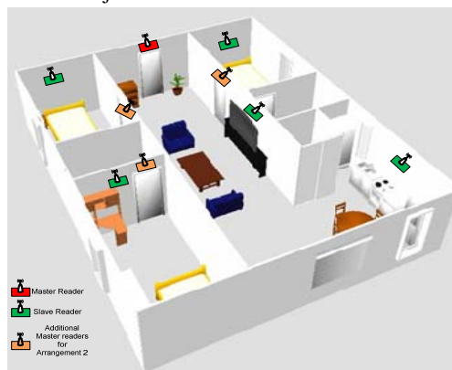
Fig 4 Arrangement of RFID Tags in Sweet Home
